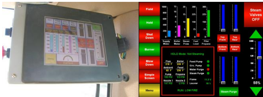
Figure 5. Control unit installed in the tractor cab
