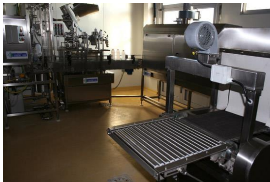
Figure 4. Part of the dairy production plant - bottled product packaging line
