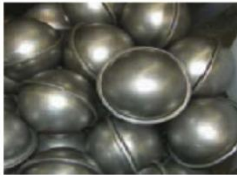
Figure 14 PCM encapsulated in metal balls 26.
