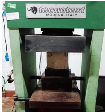
Fig. 4 Compression test on a concrete brick reinforced with natural fibers
