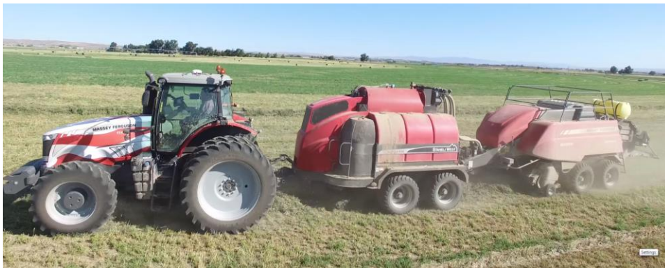
Figure 1. Position of water vapor production device between tractor and press
