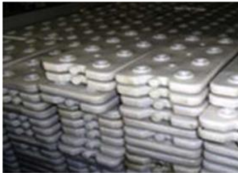
Figure 12 Commercial rectangular macro-encapsulated PCM 25.
