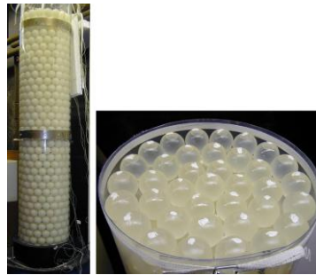
Figure 13 PCM encapsulated in spheres 26.
