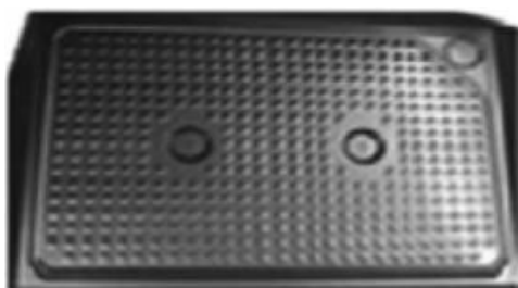
Figure 15 PCM encapsulated in aluminum panel 26.
