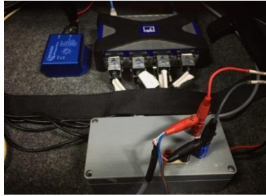
Fig. 13: Power supply, acquisition and GPS sensor located in the trunk of the vehicle
