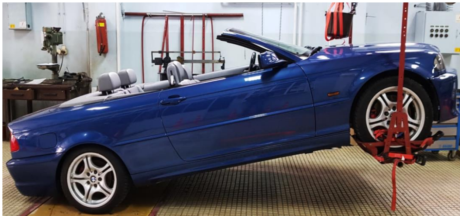
Fig. 10: Determining the height of the center of gravity
