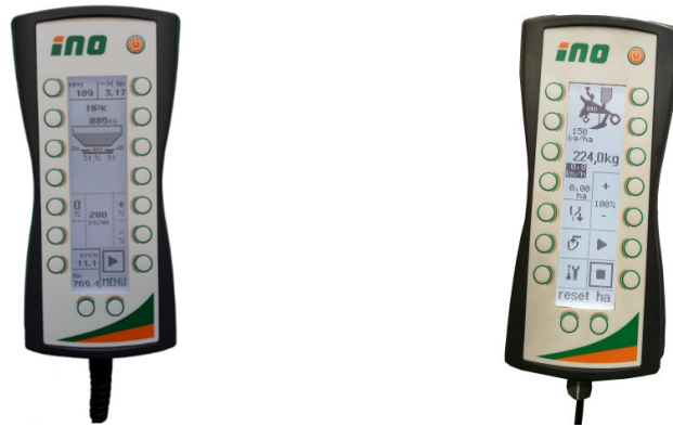
Fig. 3 Innovations from INO's Electronic Development Laboratory - INO SmartAssist for FERTI-2 Fertilizer Spreader and for VVP 115 Vibrational Subsoiler with deep fertilizer device
