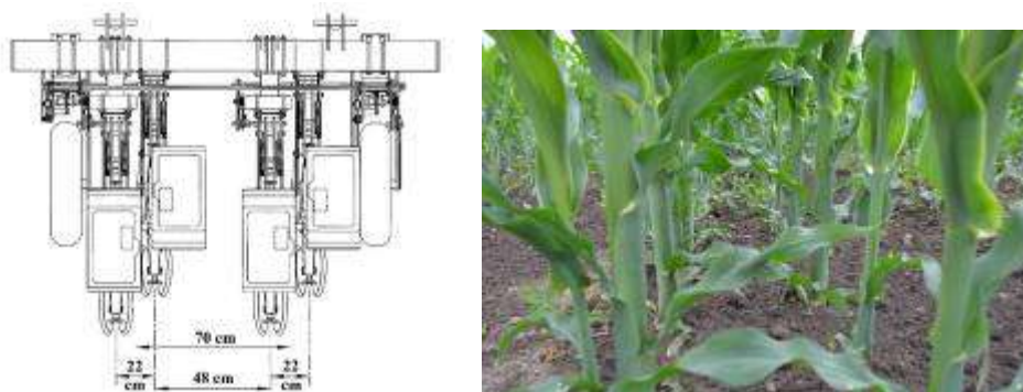
Fig. 1The basic technical features of MaterMacc twin row seeder sections
