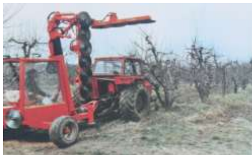
Fig. 1. Pruning machine HR-85 in operation
