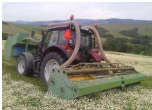
Fig. 2 New chamomile flowers harvester, mounted on the tractor VALTRA N 123.
